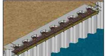
FIX PLYWOOD TO BRACKETS TO CONSTRUCT WORKING PLATFORM/SOFFIT FOLLOWED BY FIXING HANDRAIL.
